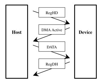
Figure 5.17 DMA data-out command protocol
